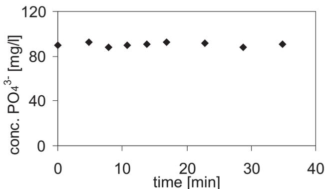
Fig. 3: Time dependence of the  $\text{PO}_4^{3-}$  concentration in the output SBF solution during exposure of silica glass granulate
