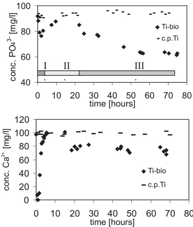
Fig. 2: Time dependence of the  $\text{PO}_4^{3-}$  and  $\text{Ca}^{2+}$  concentration in the output SBF solution during exposure of Ti-bio and c.p.Ti sample, indicating three phases of interaction
