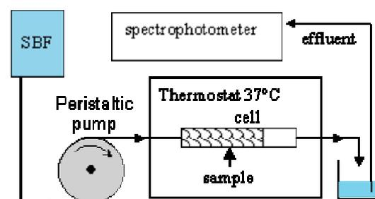
Fig. 1: Experimental arrangement of the flow-through SBF test
