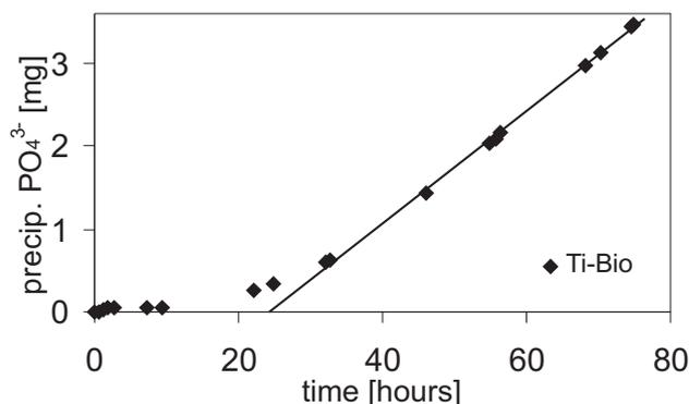
Fig. 7: Time dependence of the precipitated  $\text{PO}_4^{3-}$  weight plotted for Ti-Bio sample
