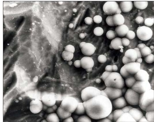
Fig. 5: SEM image of apatite crystals formed on the surface of Ti-bio sample after 74 hours of dynamic exposure in SBF (magn: 1000x)
