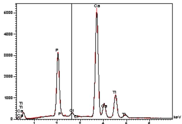
Fig. 6: EDS analysis of apatite crystals formed on the surface of Ti-Bio sample after 74 hours of dynamic exposure in SBF
