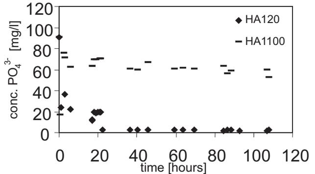
Fig. 4: Time dependence of the  $\text{PO}_4^{3-}$  and Ca concentration in the output SBF solution during exposure of HA120 and HA1100 samples
