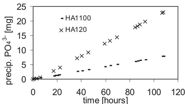
Fig. 8: Time dependence of the precipitated  $\text{PO}_4^{3-}$  weight plotted for HA120 and HA1100
